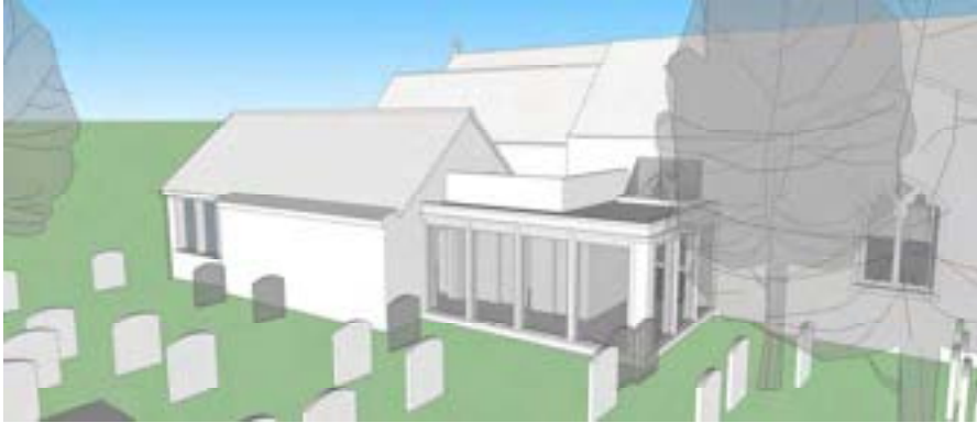
Discounted Option B - MVHR unit placed on top of Pentice roof with external screening up to 1m high to perimeter of equipment.
