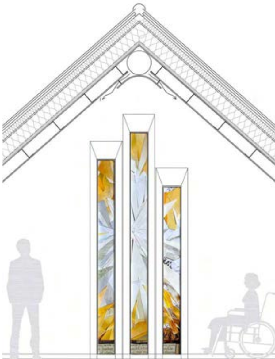
Extract of Section F-F showing the East gable-wall window design. Three slender stained glass windows forming one artistic composition, integrated into the architectural language of the new extension and into the wider context of the Church and Churchyard.
