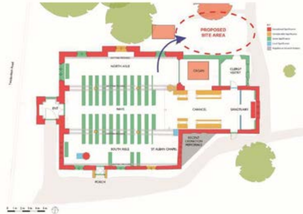
OPTION FOR NEW CONNECTION BETWEEN CHURCH AND EXTENSION A: Through North Aisle (Preferred)
