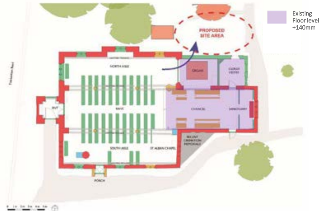
OPTION FOR NEW CONNECTION BETWEEN CHURCH AND EXTENSION B: Through Organ Chamber (note: step in floor level)
