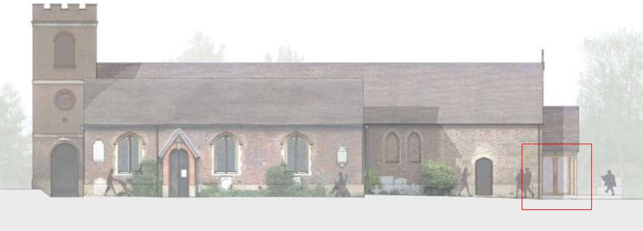
PROPOSED SOUTH ELEVATION: Recommended Option 4 – Oak framed clear glazed double door, serving the extension’s function as a community space.
