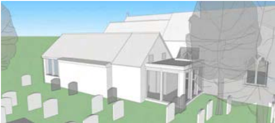
Discounted Option C - MVHR unit placed on top of Pentice roof with an extended pitched roof form to house it.
